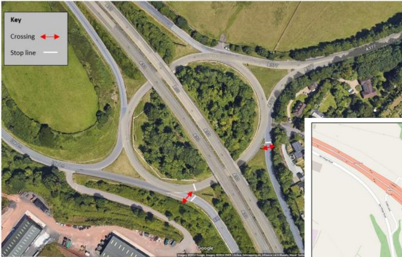
Figure 13: location of traffic lights on slip roads
